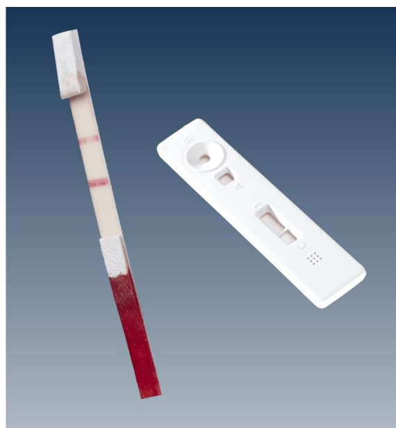
Figure 10: Lateral flow assay with sample pad that has a red blood cell filter. Image from mdimembrane.com/
