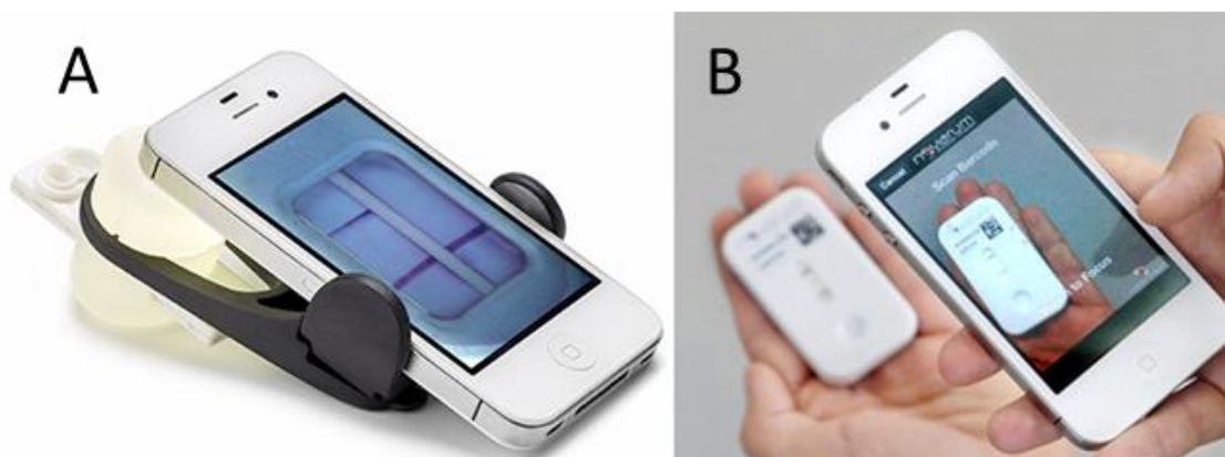
Figure 4: (A) i-calQ smartphone reader with strip holder attachment. (B) Novarum hardware-free reader.
