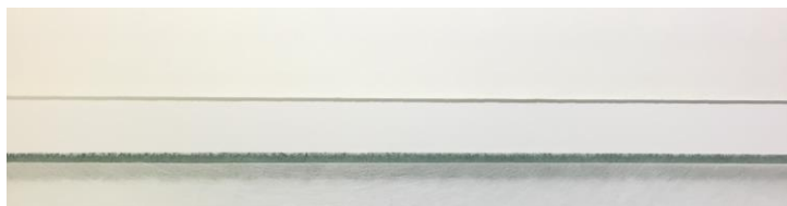
Figure 11: Assembled 30 cm master card with 150 nm Gold nanoshell conjugate. This card is subsequently cut into the final test strips orthogonal to its length
